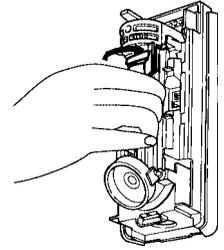
Hold the pyro electric unit and turn it to the desired direction (15° steps).
