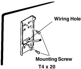
Pull the wire through wiring hole and install the plate on the wall by using provided mounting screws (two places).
