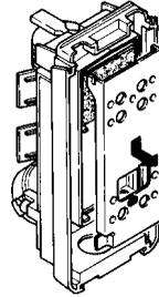
Remove the plate by sliding it down and away from the unit base.
