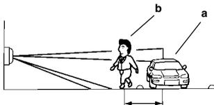
The detection area might increase when there is a big temperature difference between the moving object and the background.
