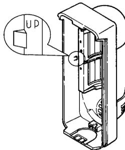
5. Place the lens holder. Confirm the lens holder is held by left and right prongs on the cover.
