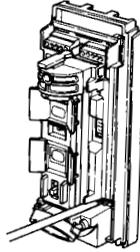
Loosen the plate lock screw [about 10mm (0.4")].
