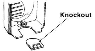
Conduit can be installed directly into the bottom of the unit by removing the knockout on the bottom on the cover.
