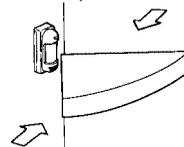
4. VX-402 is designed to protect any light disturbances. However, too much light may cause unstable condition with the sensor, such as; strong sunlight directed or reflected exactly into the sensor's field of view. It is recommended to avoid such installation.
