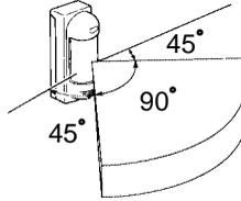
Area angle is 90° with 7 fingers by 15° Turn optical cylinder. Angle moves by 15° per notch.
