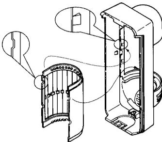
4. Put the lens back in by aligning the 4 projections on the cover to the 4 cut outs on the lens. Please do not put the lens upside down.
