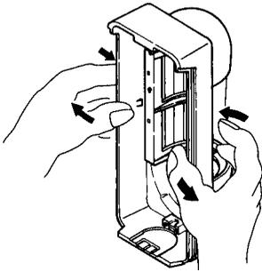
1. Remove the lens holder from the cover as shown above.
