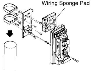
Fix bracket onto mounting plate with supplied screws (M4x6,4pcs). Place the bracket around the pole and tighten firmly with pole locking screws.
