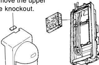
Lead the wire through the upper side of the unit base, lead the wire to the wiring slit then through the wiring hole.
