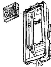
Remove the lower knockout of the unite cover, lead the wire through the knockout hole.
