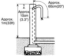
For outdoor wiring, bury piping as deep as possible. Some sites will require metal coated cables for underground wiring work. Avoid aerial wiring
