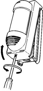
Loosen the lock screw and remove the cover.
