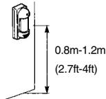
3. Mount the sensor so that a majority of traffic flow is across the detection pattern.
