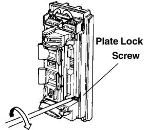
Fasten the plate lock screw and connect the wires to the terminal.
