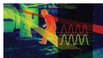
Correlated signal in both channels = PIR Alarm
